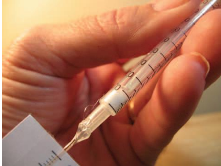
Figure 2: Inserting a cotton plug into the barrel of the constructed microrespirometer.
