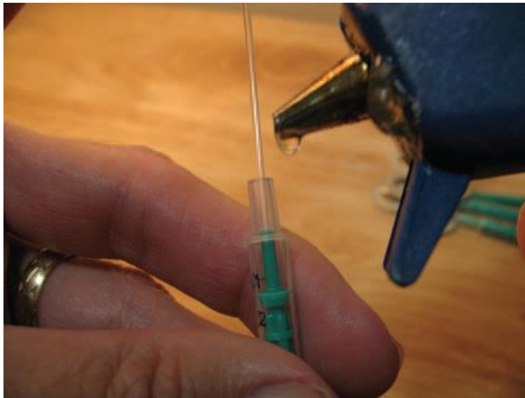
Figure 1: Adding hot glue to the base of the capillary tube.
